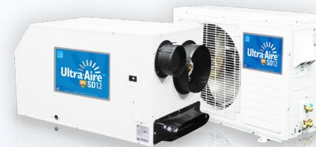
The Ultra-Aire SD12 is the first two-piece, high efficiency, split whole house ventilating dehumidifier that allows sensible heat load generated from dehumidifying the house to be released by the outdoor condensing unit.
